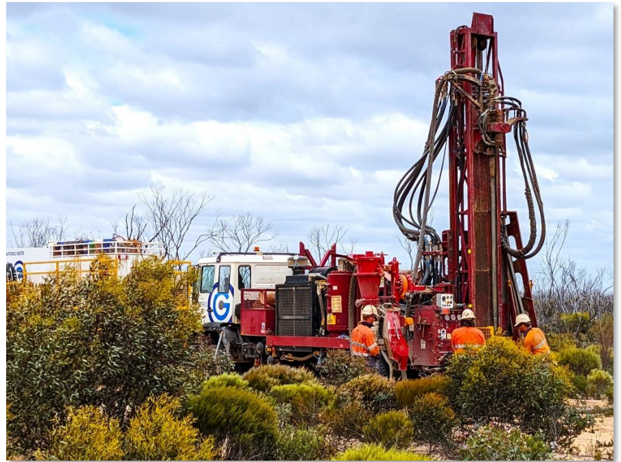
Figure 1: AC Rig on site, drilling first traverse
